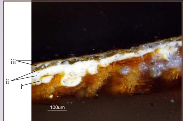
The paint analysis on the interior of the window sash indicates the windows were originally faux painted to simulate oak and subsequently repainted to simulate mahogany which is consistent with the interior window surround.
