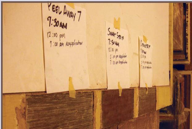
Three different solvents were tested to determine the most effective removal technique without adversely impact the wood sash.
