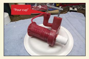
The "Lost Wax" process was used for casting the new finials. First, a pattern of the historic finial was hand carved. Using the pattern, a mold was created to make the wax castings. The funnel-shaped element and rods are a "pour cup" to allow the molten metal to be poured in and gases escape.
