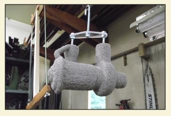
Fine aggregate (sand) is then "painted" onto the wax mold, with successive layers of more course aggregate added to create a "shell". The shell is then baked at high temperature. The wax melts leaving the shell which can then be filled with the molten metal.
