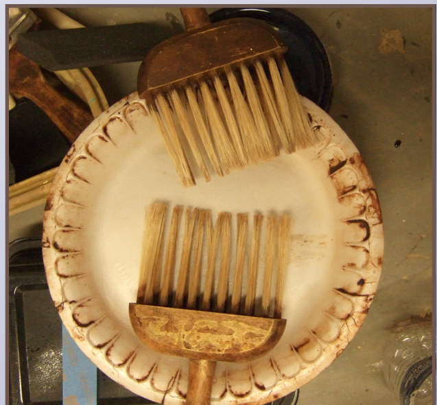
"Graining" is a faux finishing technique that uses a combination of paints and glazes to transform wood from one species to another. Wood graining tools used by the craftsman to grain the sash.
