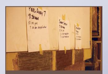
Three different solvents were tested to determine the most effective removal technique without adversely impact the wood sash.
