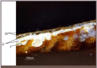
The paint analysis on the interior of the window sash indicates the windows were originally faux painted to simulate oak and subsequently repainted to simulate mahogany which is consistent with the interior window surround.
