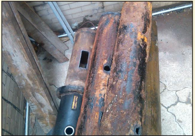
The original casing shows fissures and rust. A new steel casing with a PVC liner will be installed around the new hydraulic jack protecting the steel from corrosion. The new casing is welded together.
