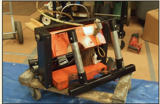
The safety device (also known as the "Jaws of Life") was removed from the jack for reinstallation on new jack. In the event of a failure, this device closes on the piston and stops the cab from falling.
