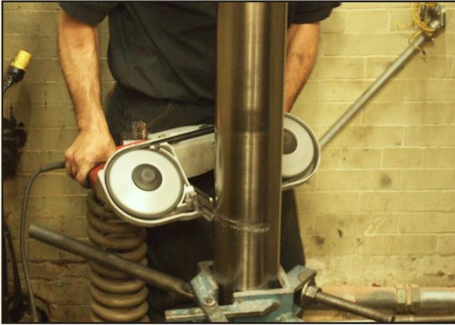
The steel jack was cut into small pieces and removed from casing. In several instances rust was visible on the jack.
